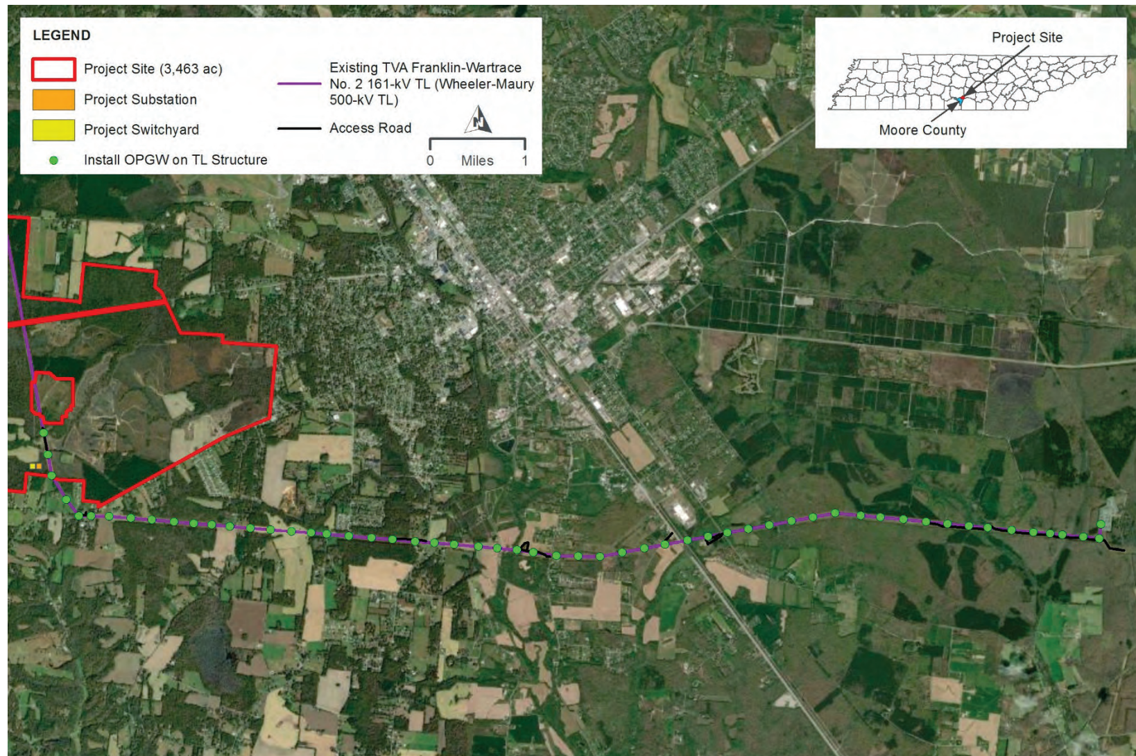
Figure 2-5. The Proposed Project Substation, Switchyard, and Work Areas Along the Existing TVA Franklin–Wartrace No. 2 161-kV TL
