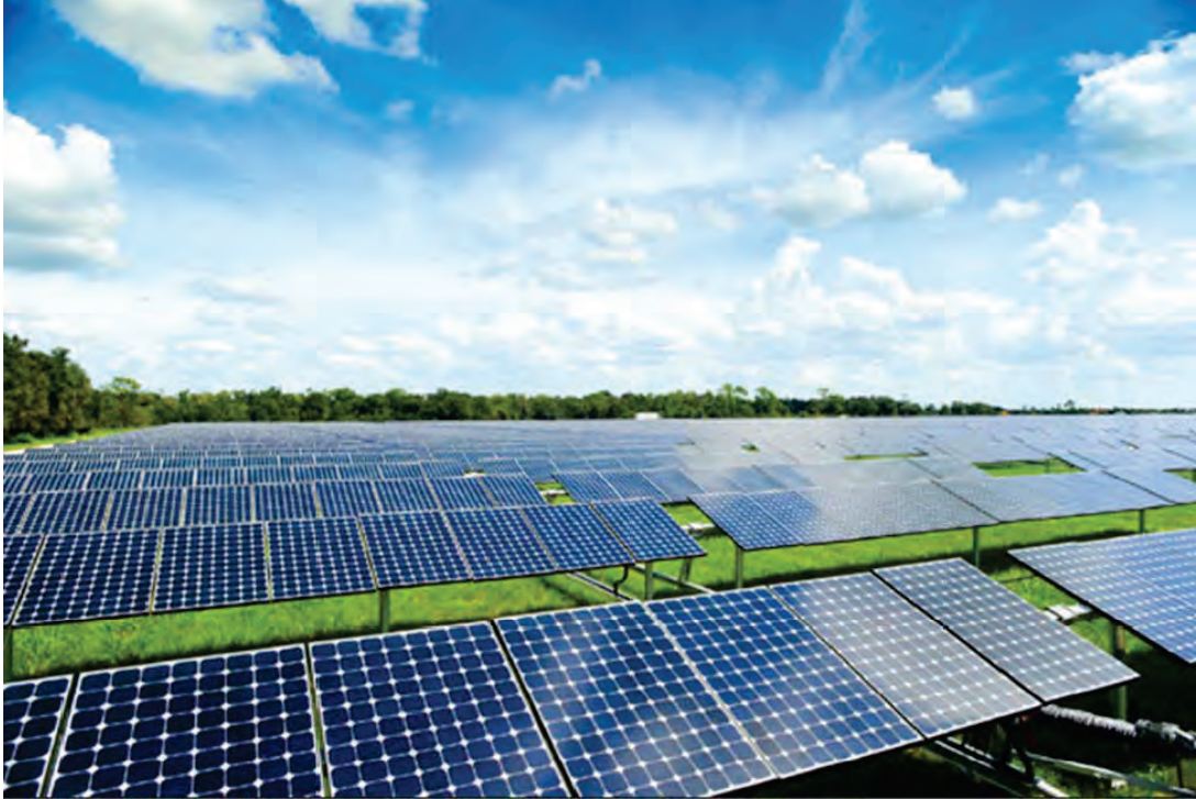
Photo 3-11. Single-axis, Tracking PV System with Panels Showing Some Tilt as Viewed from the East or West
