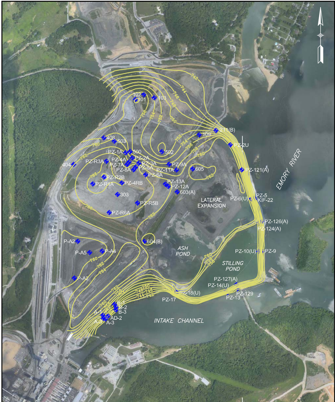
FIGURE 6 GROUNDWATER ELEVATIONS IN ASH AND SHALLOW SOILS (JULY 2010) KINGSTON ASH RECOVERY PROJECT
