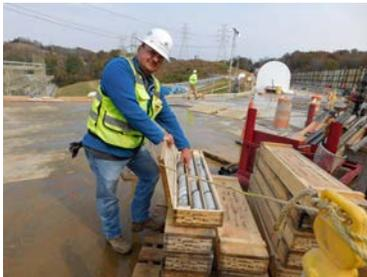
*Technical Field Lead Scott Lakes examines core samples taken during drilling on the dam's earthen embankment.*
