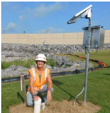
Lead Dam Safety Engineer Carol Ford checks a piezometer, which measures pressure and depth of groundwater
