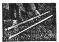
Figure 4.34. Macro-Core® liner filled with soil core.
