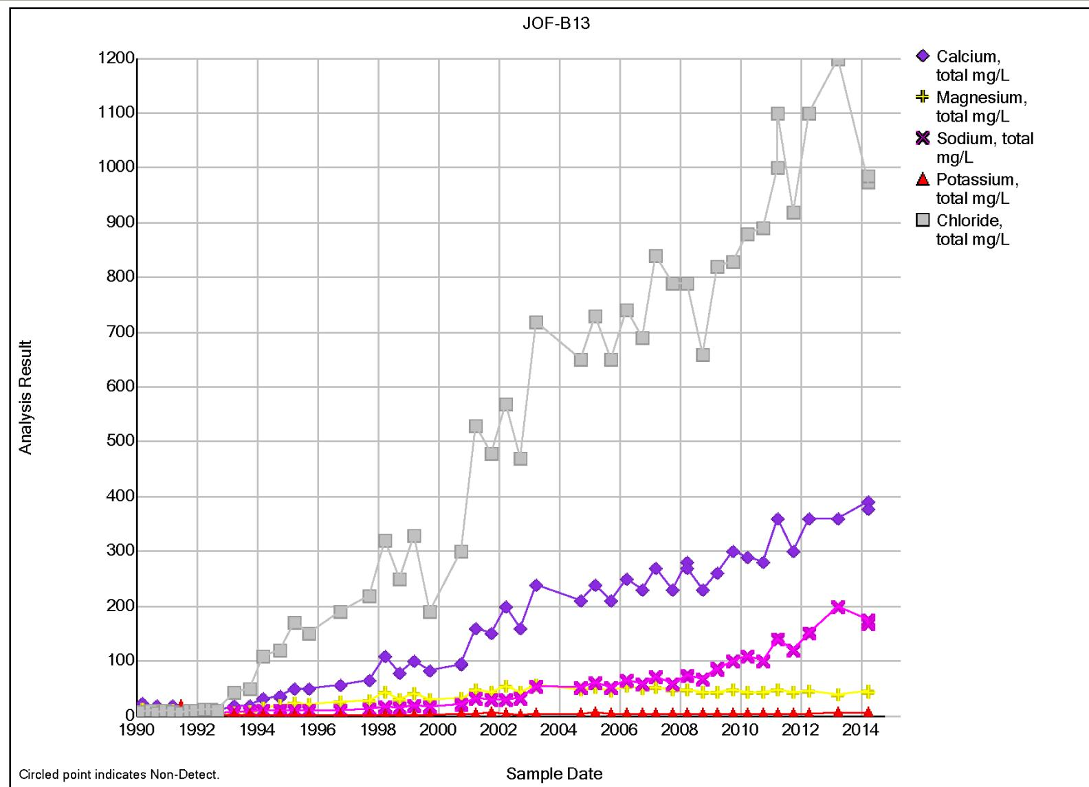
Figure 1. Chloride and Major Cation Concentration Time Series for Background Well B13 (1990 - 2014)
