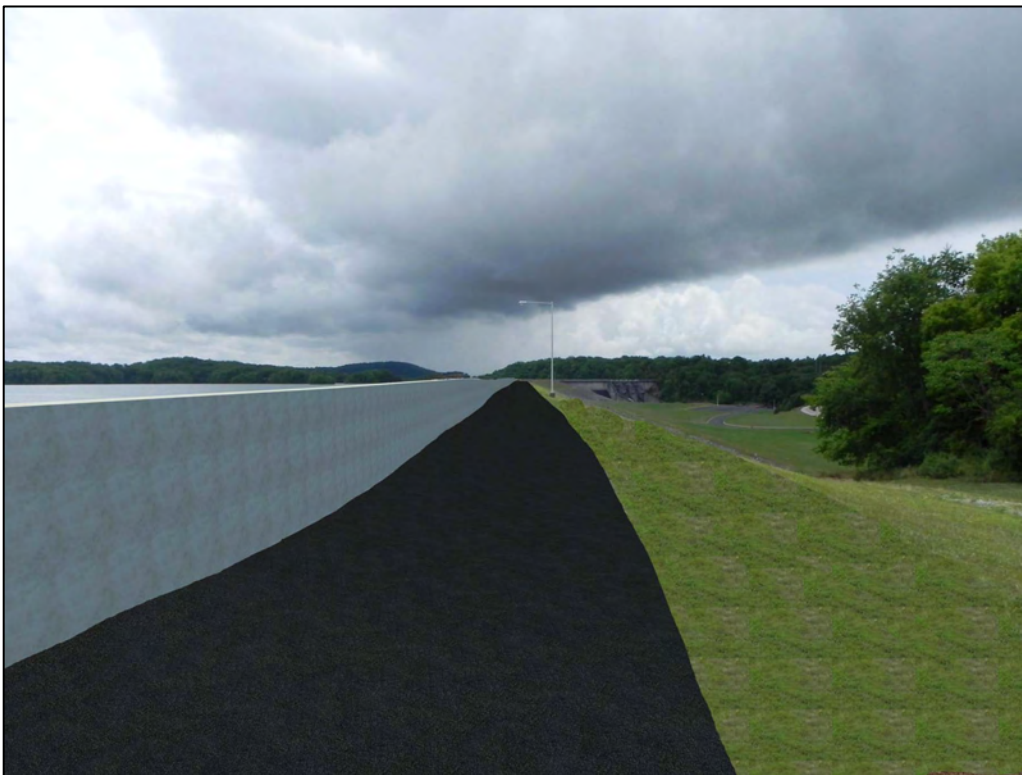
Photo 3.14-9b. Rendering of a 4.8-foot-tall Floodwall and 2-ft Raised Walkway at T-2
