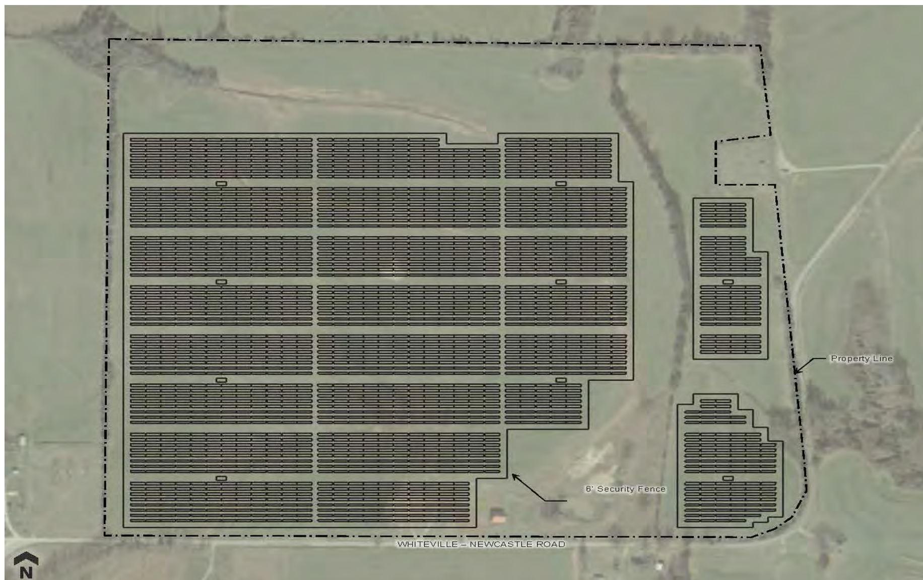
Figure 2-2. Latitude Solar Center conceptual site plan – Option 2, fixed tilt system.
