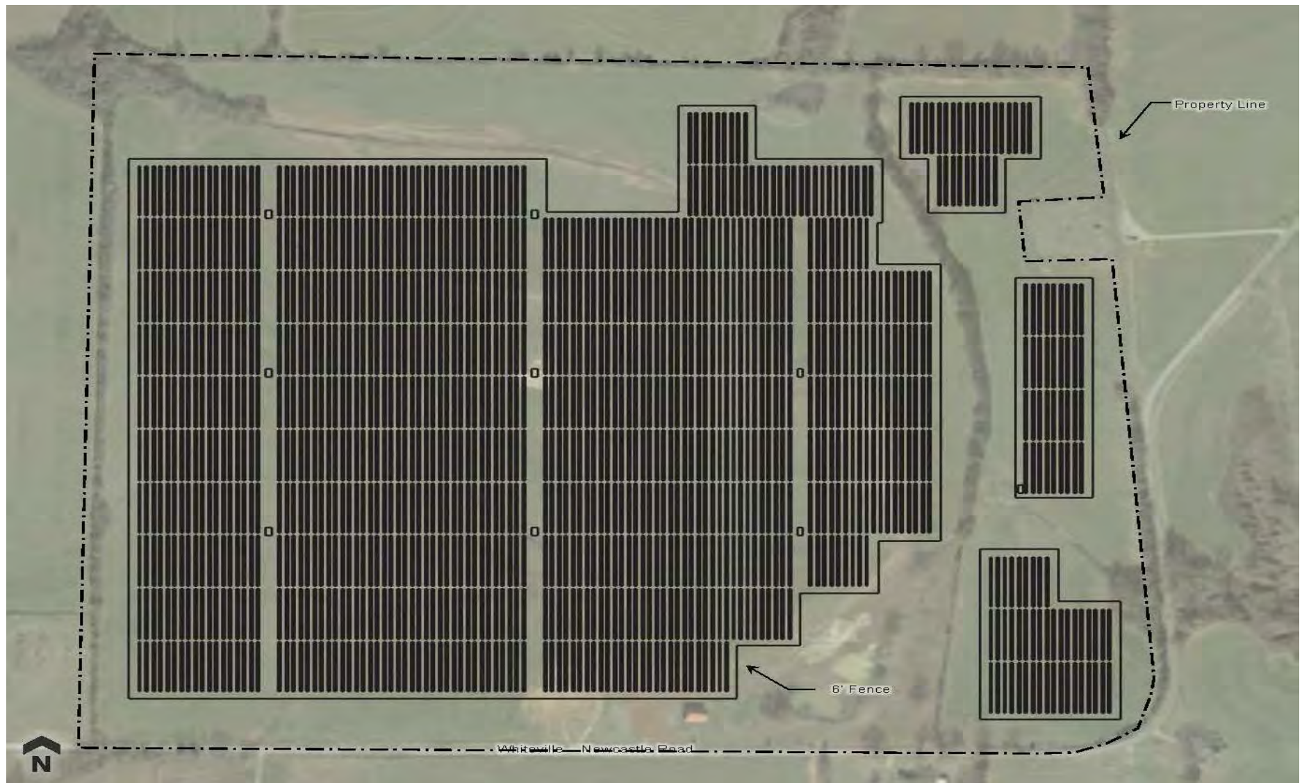
Figure 2-1. Latitude Solar Center conceptual site layout – Option 1, single-axis tracking system.
