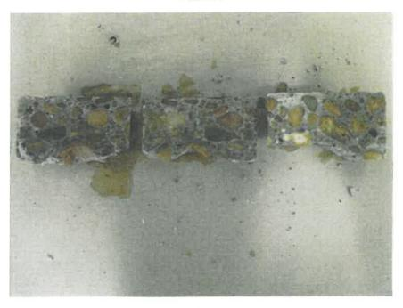
Photo 22: Longitudinally sawn sections of Core #5 from arch. No fractures are apparent.
