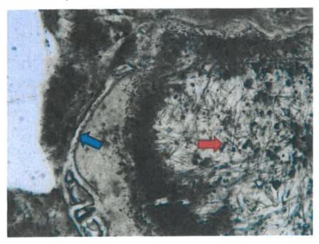
Photo 38: Photomicrograph of Core #3 from arch (Lab No. 6653) showing entrapped air void filled with ettringite (red arrow) and microfractures (blue arrow). Plane polarized light, magnification 200X.
