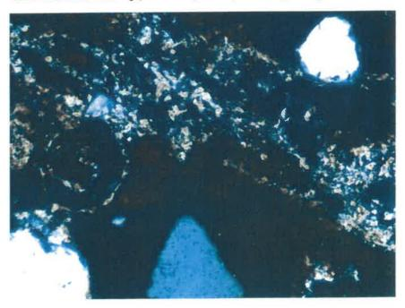
Photo 40: Photomicrograph of Core #3 from arch (Lab No. 6653) showing carbonation isolated to microfractures. Crossed polars, magnification 100X.
