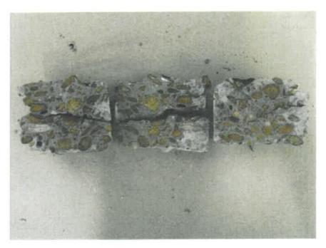
Photo 20: Longitudinally sawn sections of Core #3 from arch showing subparallel fractures normal to the core axis, likely from freeze/thaw distress.
