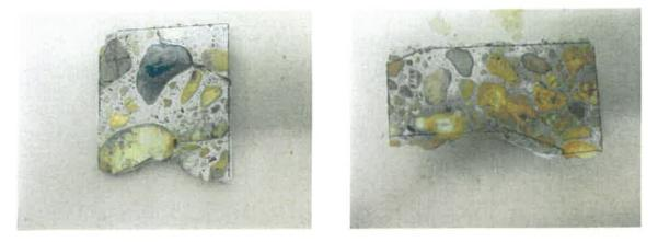
Photo 26: Sawn surfaces of Core #4 from arch (Lab No. 6654) (left) and Core #5 from arch (Lab No. 6655) (right) after application and rinsing of Los Alamos stains. No ASR is apparent.
