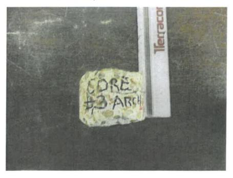
**Photo 8**: Core #3 from arch (Lab No. 6653), as received. Note subparallel fracturing likely due to freeze-thaw distress.
