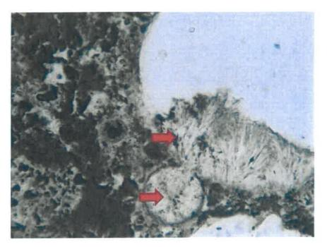
Photo 30: Thin-section photomicrograph of Core #3 from bridge deck (Lab No. 6650) showing ettringite needles in matrix and air voids (red arrows). Plane polarized light, magnification 200X.
