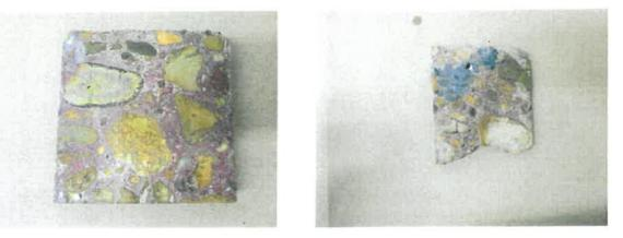
Photo 28: Sawn surfaces of Cores Core #1 from arch (Lab No. 6652) (left) and Core #3 from arch (Lab No. 6653) (right) after application of phenolphthalein stain. Areas not stained magenta are carbonated.
