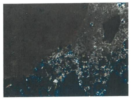
Photo 35: Photomicrograph of Core #4 from bridge deck (Lab No. 6651) showing carbonated (top) and non-carbonated (bottom) matrix. Crossed polars, magnification 100X.
