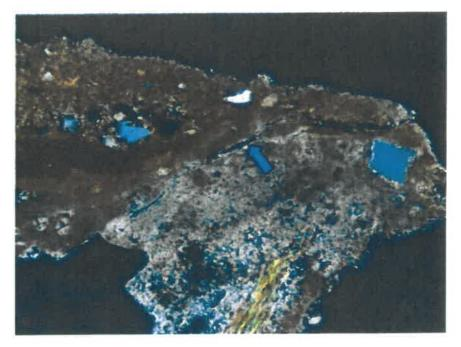
Photo 45: Photomicrograph of Core #5 from arch (Lab No. 6655) showing exterior surface carbonation and microfracture (blue arrow). Crossed Polars, magnification 100X.
