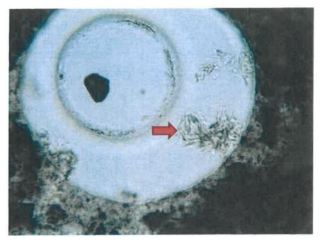
Photo 41: Photomicrograph of Core #4 from arch (Lab No. 6654) showing entrapped air void containing ettringite needles (red arrow). Plane polarized light, magnification 400X.
