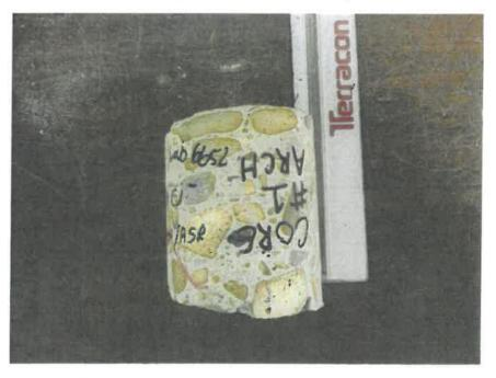
Photo 6: Core #1 from arch (Lab No. 6652), as received.
