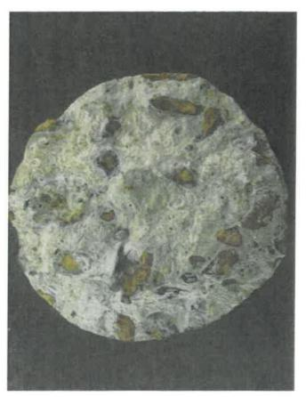
Photo 10: Interior surface of Core 3 from arch; showing possible carbonate deposits (white) around aggregate particles.
