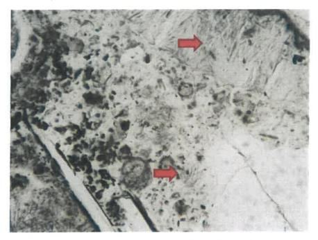
Photo 31: Thin-section photomicrograph of Core #3 from bridge deck (Lab No. 6650) showing ettringite needles in the paste of the concrete. Plane polarized light, magnification 200X.
