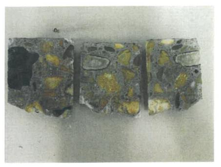
Photo 19: Longitudinally sawn sections of Core #1 from arch. No fractures are apparent, but "rinds" around coarse aggregate particles are evident.
