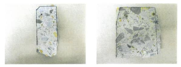
Photo 24: Sawn surfaces of Core #3 from bridge deck (Lab No. 6650) (left) and Core #4 from bridge deck (Lab No. 6651) (right) after application and rinsing of Los Alamos stains. No ASR is apparent.
