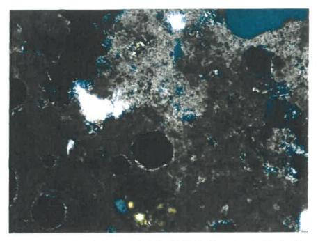
Photo 43: Photomicrograph of Core #4 from arch (Lab No. 6654) showing carbonated (top) and non-carbonated (bottom) matrix. Crossed polars, magnification 100X.
