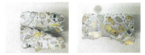
Photo 29: Sawn surfaces of Core #4 from arch (Lab No. 6654) (left) and Core #5 from arch (Lab No. 6655) (right) after application of phenolphthalein stain. Areas not stained magenta are carbonated.
