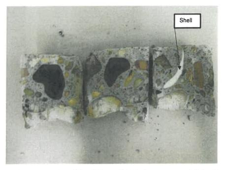
Photo 21: Longitudinally sawn sections of Core #4 from arch. No fractures are apparent. Note white arcuate shell fragment.
