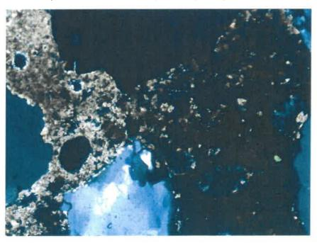
Photo 32: Photomicrograph of Core #3 from bridge deck (Lab No. 6650) showing carbonated (left) and noncarbonated (right) matrix. Crossed polars, magnification 100X.
