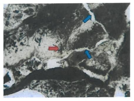
Photo 39: Photomicrograph of Core #3 from arch (Lab No. 6653) showing ettringite present in paste (red arrow) and associated microfracturing (blue arrows). Plane polarized light, magnification 200X.
