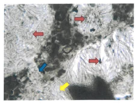
Photo 33: Photomicrograph of Core #4 from bridge deck (Lab No. 6651) showing ettringite needles in paste (yellow arrow), microfracting (blue arrow) and air voids (red arrows). Plane polarized light, magnification 400X.
