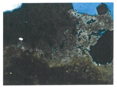
Photo 37: Photomicrograph of Core #1 from arch (Lab No. 6652) showing carbonated (top) and non-carbonated (bottom) matrix. Crossed polars, magnification 100X.
