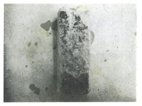
Photo 3: Fractured side of Core #3 from bridge deck.
