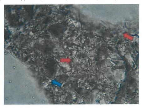
Photo 34: Photomicrograph of Core #4 from bridge deck (Lab No. 6651) showing ettringite needles in paste (red arrows) associated with microfracturing (blue arrow). Plane polarized light, magnification 600X.
