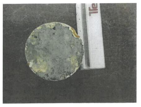
Photo 15: Top surface of Core #5 from arch, as received
