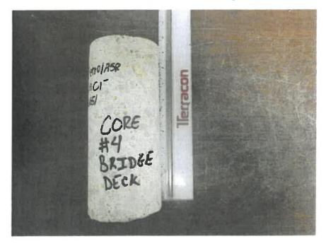
Photo 4: Core #4 from bridge deck (Lab No. 6651), as received.
