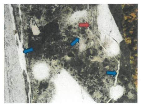
Photo 42: Photomicrograph of Core #4 from arch (Lab No. 6654) showing exterior surface microfractures (blue arrows) and ettringite in paste (red arrow). Plane polarized light, magnification 100X.
