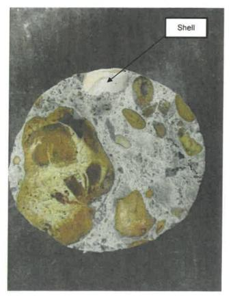
Photo 12: Bottom surface of Core #4 from arch showing large aggregate and shell (white).
