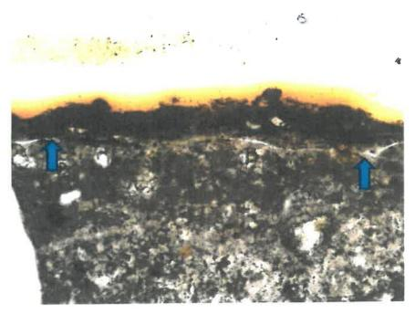
Photo 36: Photomicrograph of Core #1 from arch (Lab No. 6652) showing carbonation of exterior surface and microfracturing parallel to the exterior surface. Plane polarized light, magnification 100X.
