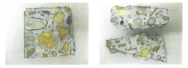
Photo 25: Sawn surfaces of Cores Core #1 from arch (Lab No. 6652) (left) and Core #3 from arch (Lab No. 6653) (right) after application and rinsing of Los Alamos stains. No ASR is apparent.
