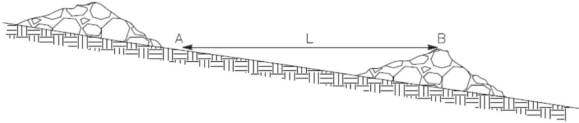
DETAIL: SPACING BETWEEN CHECK DAMS
