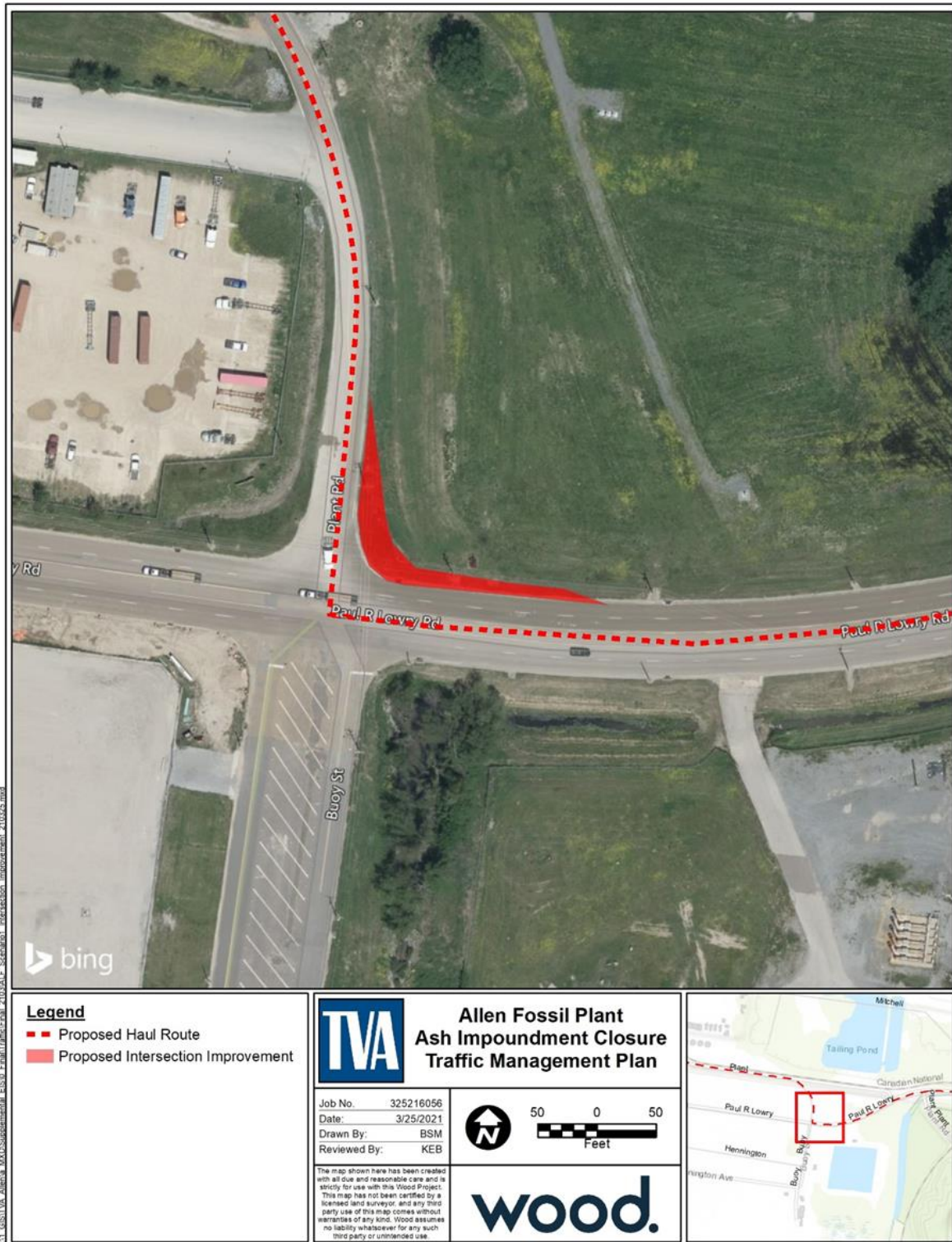
Figure 4-3. Proposed Plant Road Right Turn Improvement for Current Access Route to ALF
