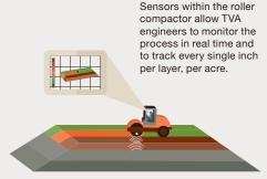
The data that the sensors detect helps to identify areas that require more compaction to reach the required density.
