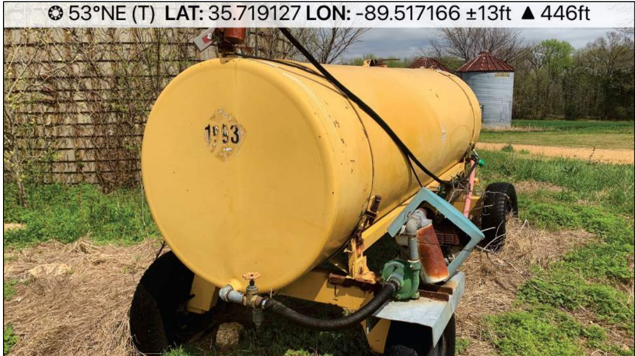
Photo 17 Mobile diesel AST.
