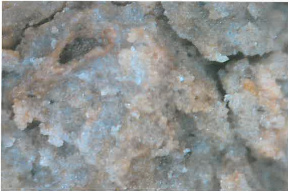
Figure 5: Representative soil at Point 2, T3S transect and microphotograph of rootlet cast formed by iron mineralization.
