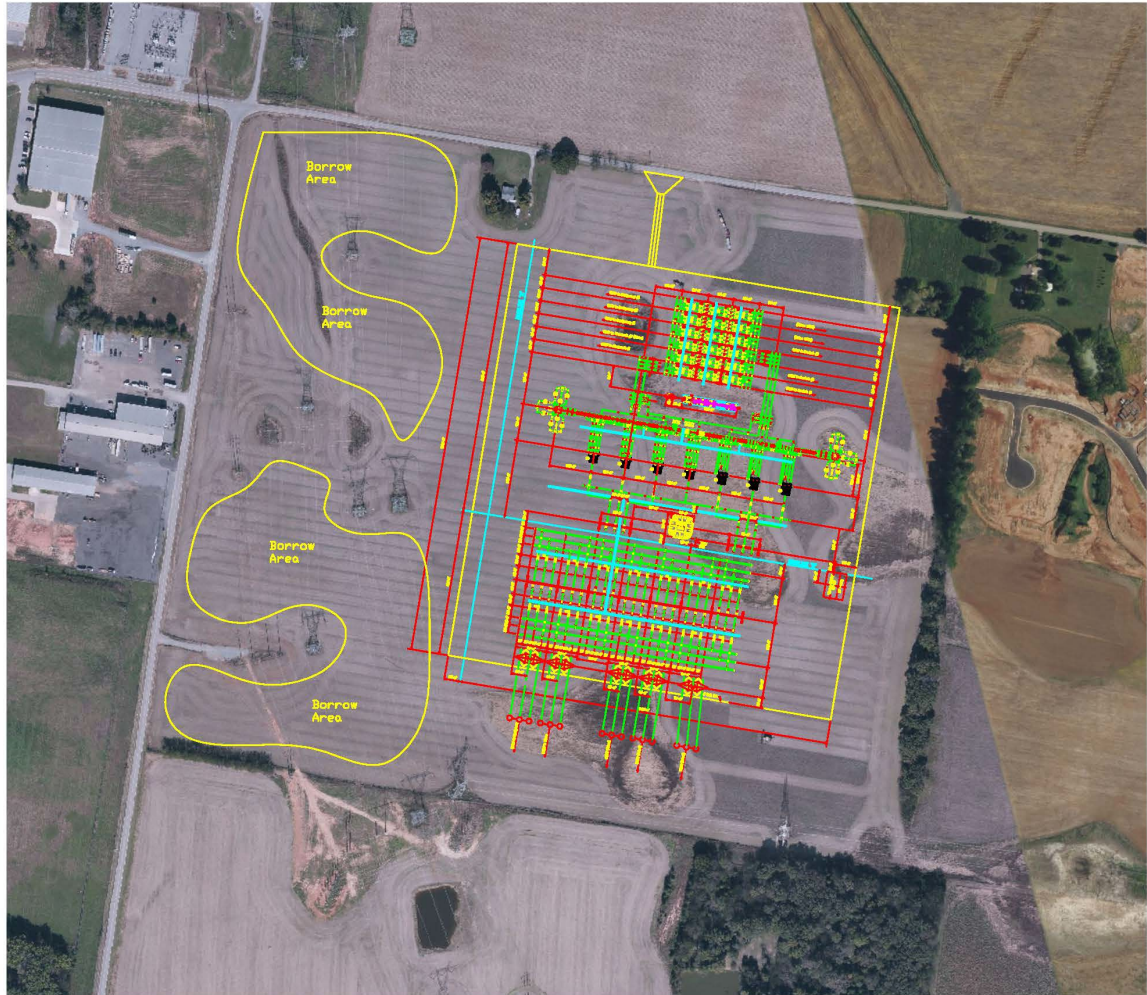
Figure 2-1. Proposed Substation Parcel Showing the Hampton Station 500-kV Substation Footprint and Designated Borrow Areas
