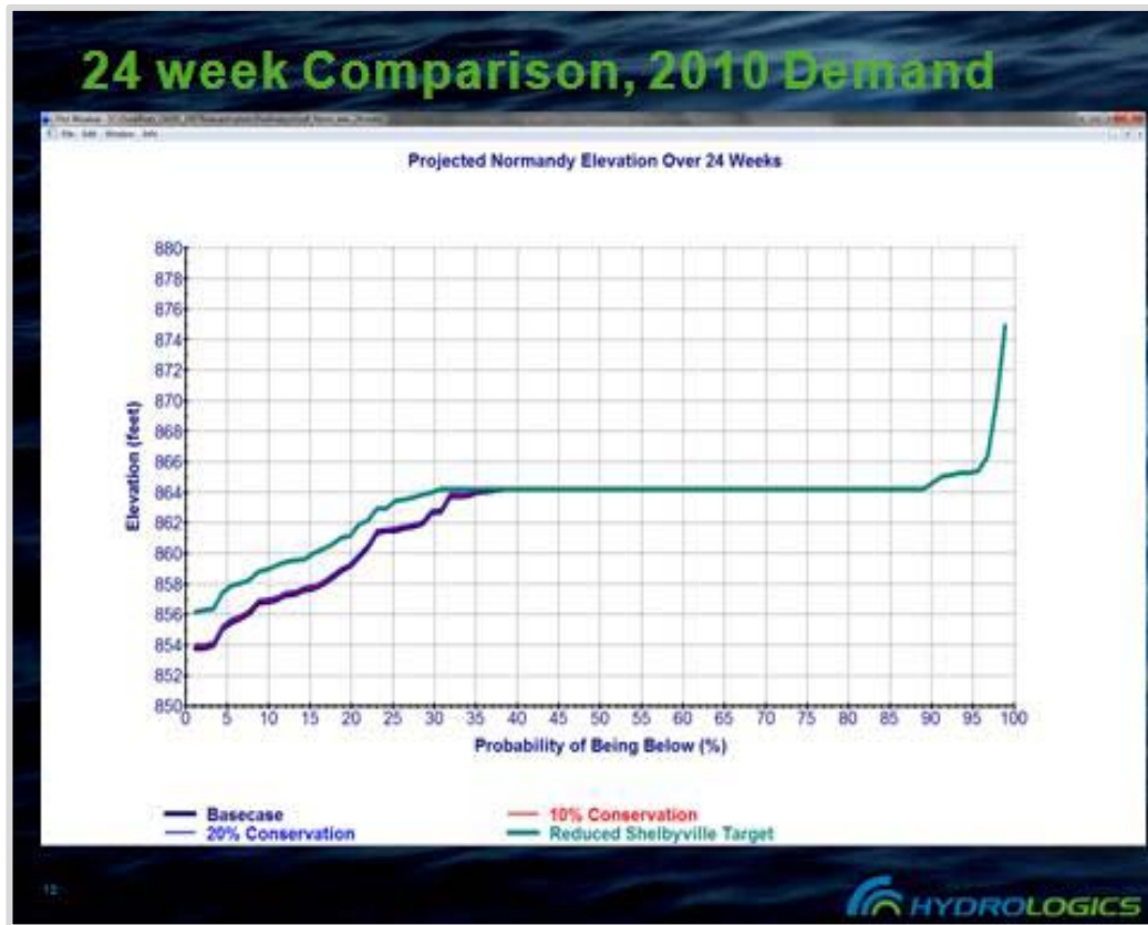
Figure 6. Impact of reduction of Shelbyville flow target and water use restrictions on Normandy Reservoir
