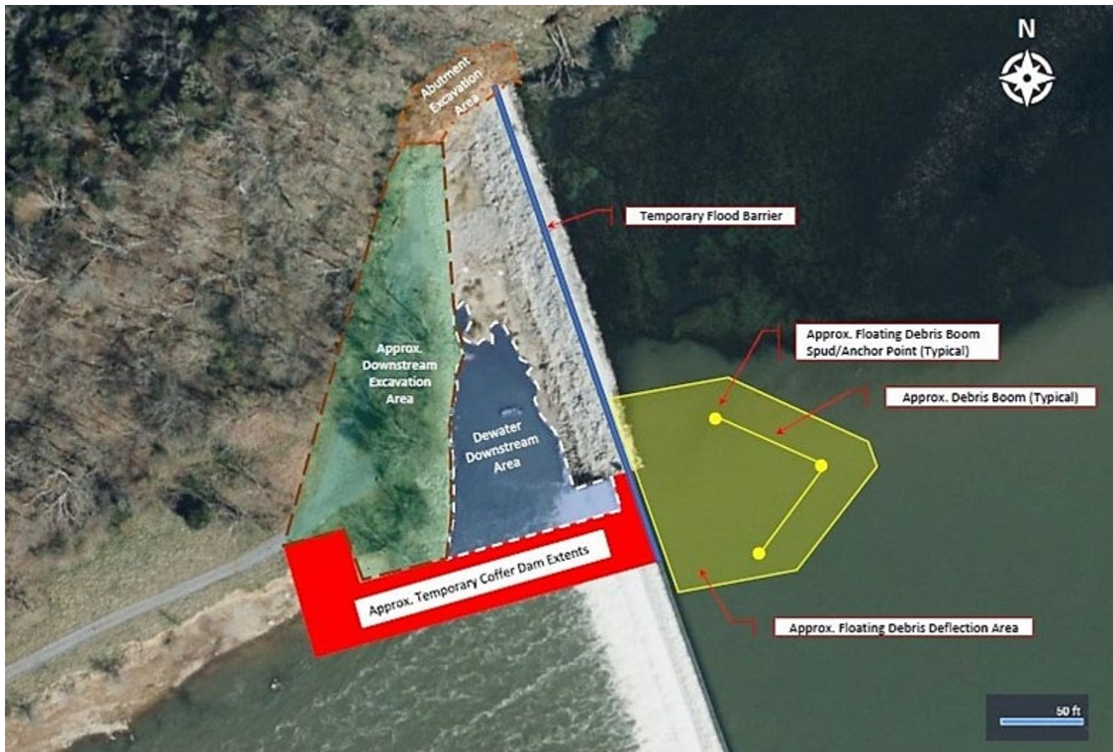
Figure 2.1-6. General Illustration of Proposed Water Control and Diversion Measures and Excavation Areas for Alternative B of the JSF Dam Modification Project (aerial image from Bing Maps)
