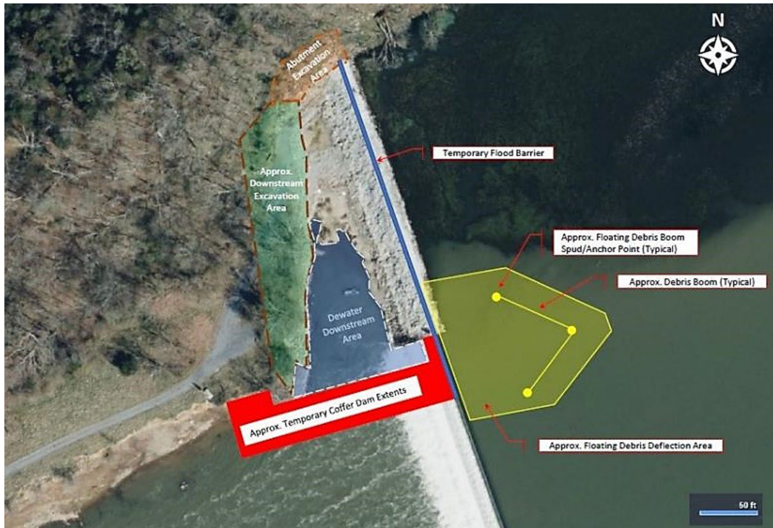
Figure 2.1-11. General Illustration of Proposed Water Control and Diversion Measures and Excavation Areas for Alternative C of the JSF Dam Modification Project (aerial image from Bing Maps)
