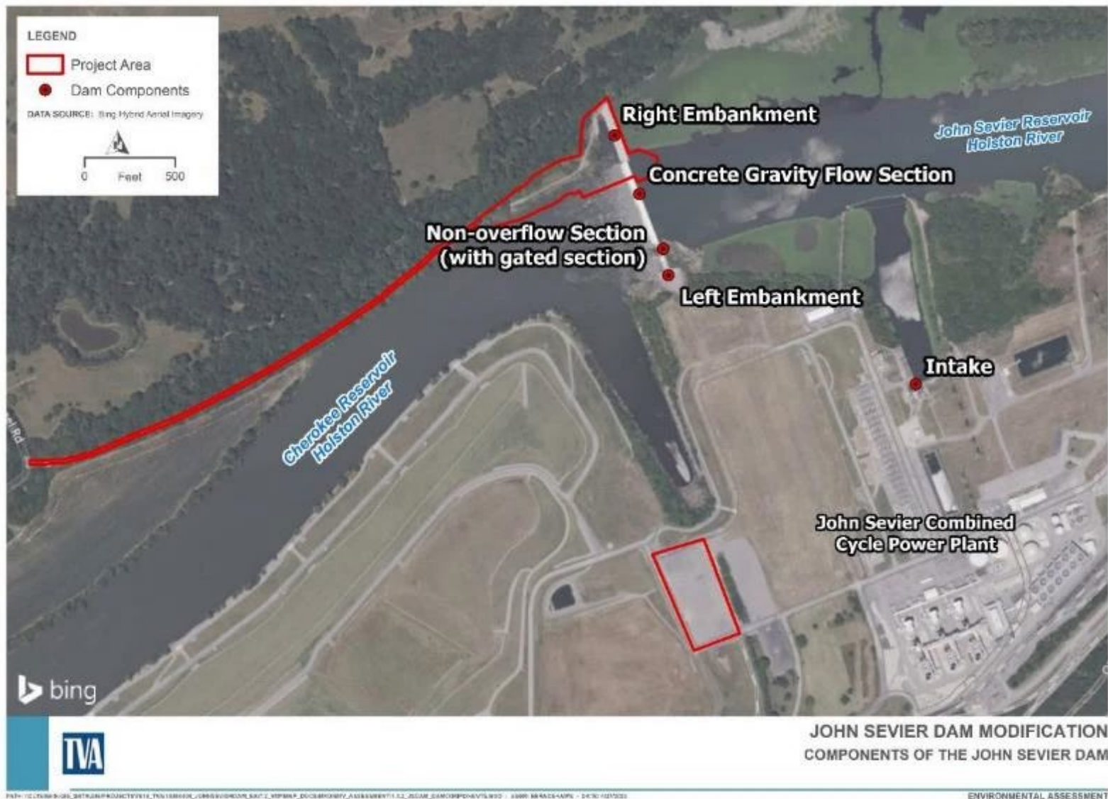
Figure 1.1-2. JSF Dam Modification Project Area and Components
