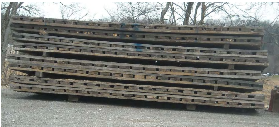
Figure 3-11. Matting Used Over Unpaved Areas for Overnight Parking
