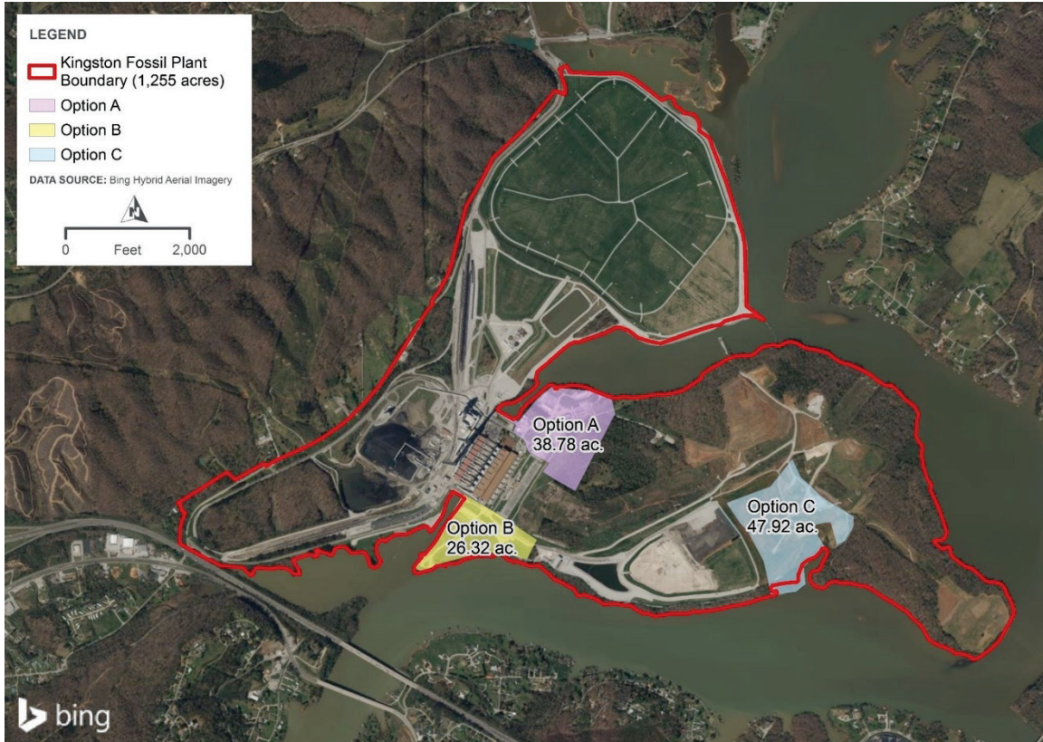
Figure 2.1-4. Alternative Siting Options Considered for the Combined Cycle/Aero Combustion Turbine Plant Proposed on the Kingston Reservation Under Alternative A
