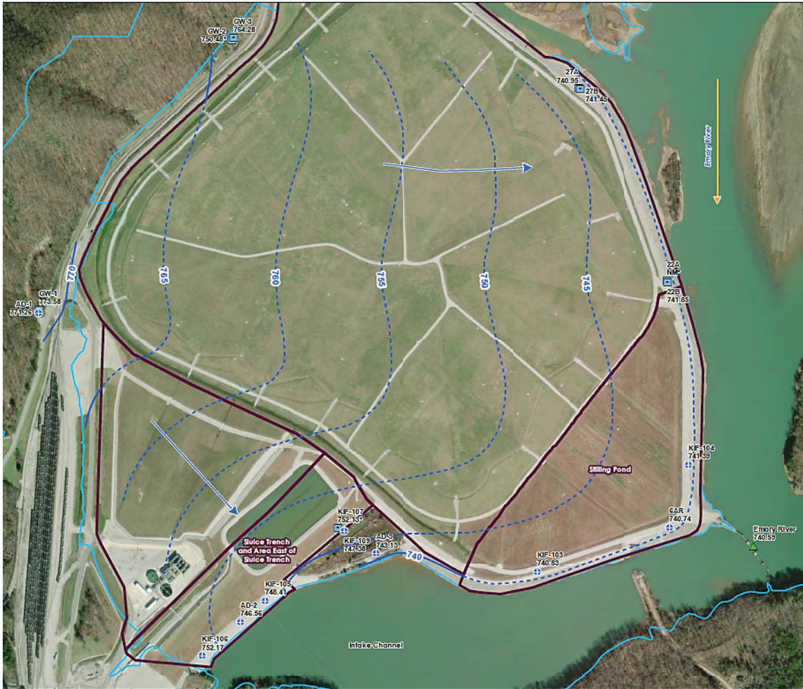
Figure 3.6-1a. Groundwater Monitoring Wells on the Kingston Reservation
