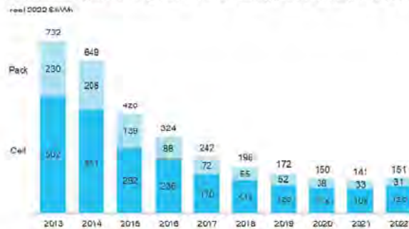
Figure 1: Volume-weighted average lithium-ion battery pack and cell price split, 2013-2022
