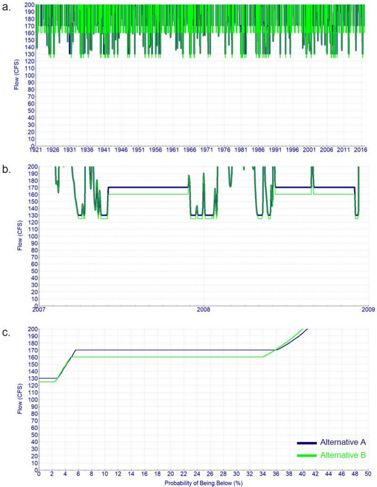
Figure B-1, Simulated flows at the Shelbyville USGS gage (03597860): (a) Simulated flow (cfs) for Alternative A and Alternative B based on the long-term hydrologic record (1921 to 2016) with recent water demands. (b) Simulated flow from 2007 to 2009 for Alternative A and Alternative B with recent water demands. (c) Probabilities of Duck River flow (cfs) based on the number of days in the historic hydrologic record for Alternative A and Alternative B with recent water demands.
