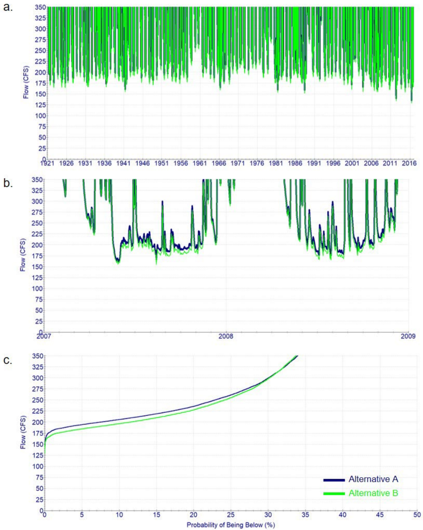
Figure B-3, Simulated flows at the USGS gage above Milltown (03599240): (a) Simulated flow (cfs) for Alternative A and Alternative B based on the long-term hydrologic record (1921 to 2016) with recent water demands. (b) Simulated flow from 2007 to 2009 for Alternative A and Alternative B with recent water demands. (c) Probabilities of Duck River flow (cfs) based on the number of days in the historic hydrologic record for Alternative A and Alternative B with recent water demands.
