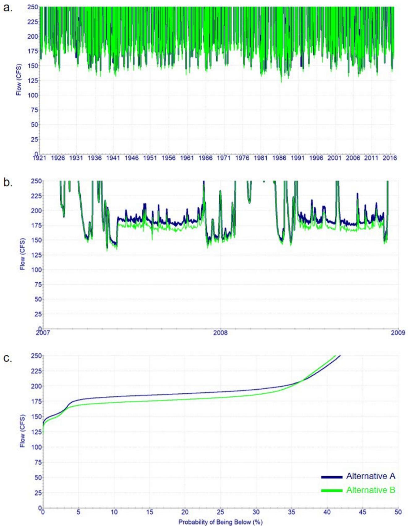
Figure B-2, Simulated flows at the USGS gage near Shelbyville (03598000): (a) Simulated flow (cfs) for Alternative A and Alternative B based on the long-term hydrologic record (1921 to 2016) with recent water demands. (b) Simulated flow from 2007 to 2009 for Alternative A and Alternative B with recent water demands. (c) Probabilities of Duck River flow (cfs) based on the number of days in the historic hydrologic record for Alternative A and Alternative B with recent water demands.
