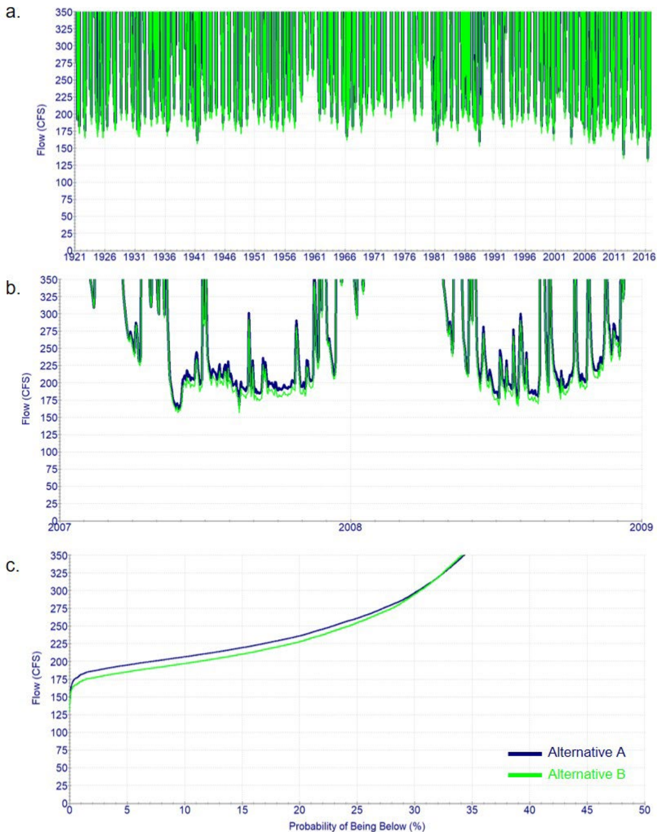
Figure B-10, Simulated flows at the USGS gage above Milltown (03599240): (a) for Alternative A and Alternative B based on the long-term hydrologic record (1921 to 2016) for future water demands. (b) Simulated flow from 2007 to 2009 for Alternative A and Alternative B with future water demands. (c) Probabilities of Duck River flow (cfs) based on the number of days in the historic hydrologic record for Alternative A and Alternative B with future water demands.
