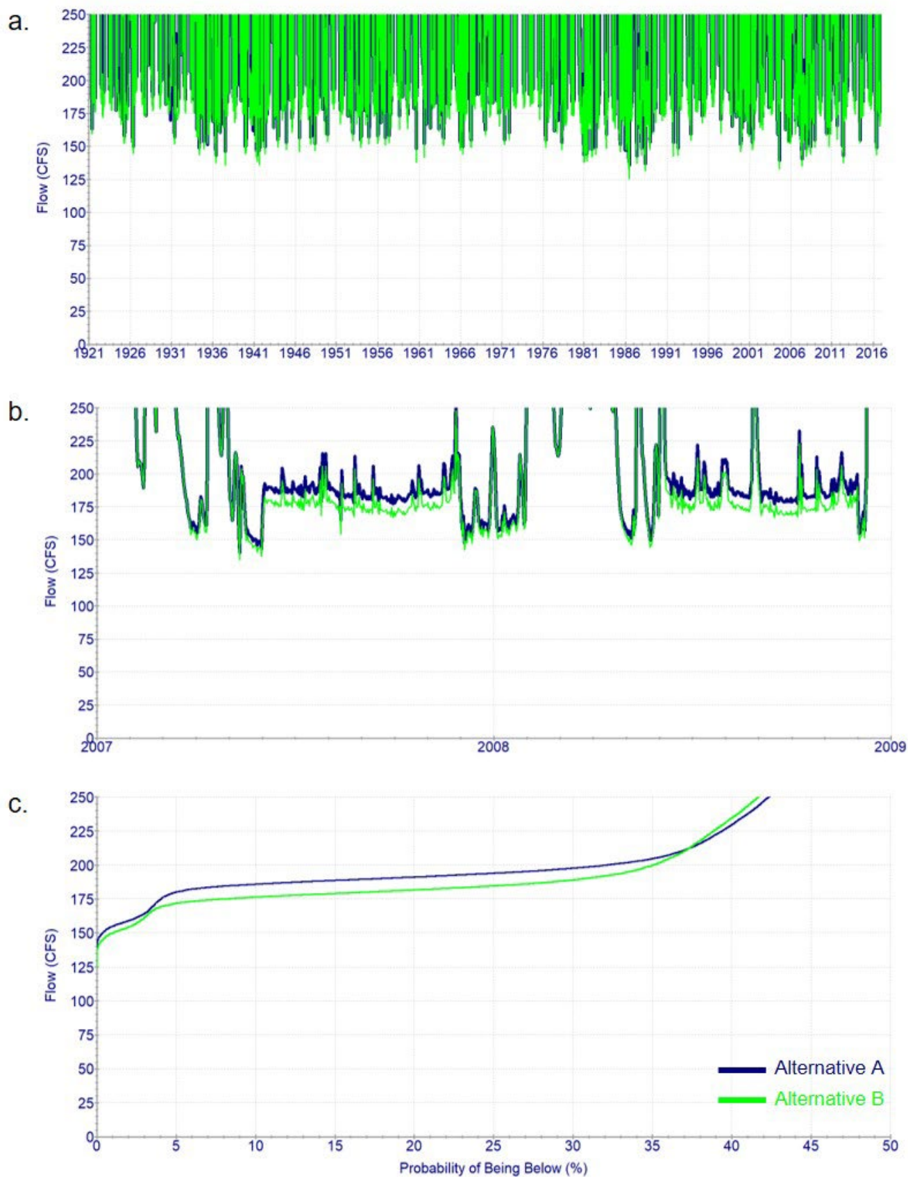
Figure B-9, Simulated flows at the USGS gage near Shelbyville (03598000): (a) Simulated flow (cfs) for Alternative A and Alternative B based on the long-term hydrologic record (1921 to 2016) with future water demands. (b) Simulated flow from 2007 to 2009 for Alternative A and Alternative B with future water demands. (c) Probabilities of Duck River flow (cfs) based on the number of days in the historic hydrologic record for Alternative A and Alternative B with future water demands.
