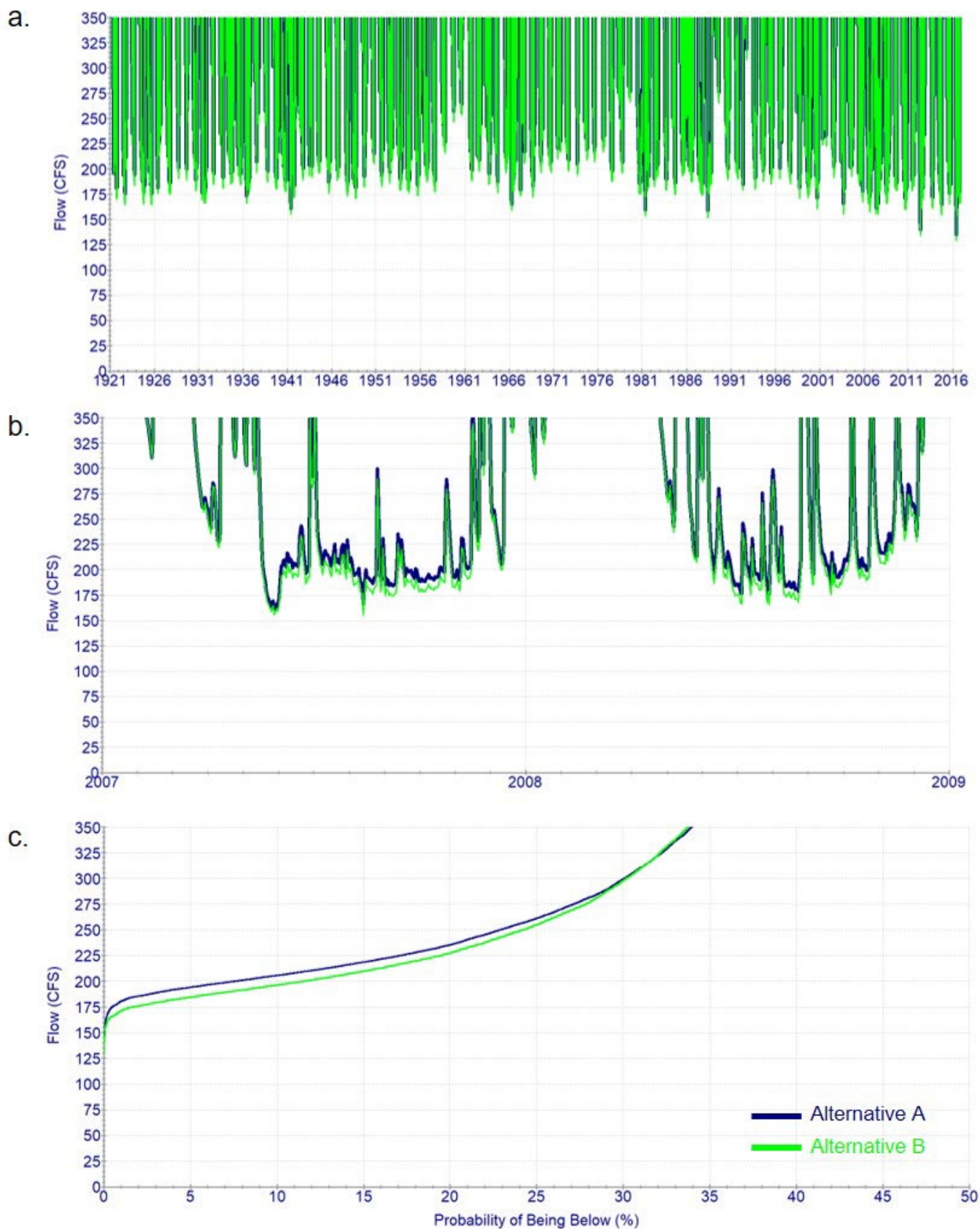
Figure B-3, Simulated flows at the USGS gage above Milltown (03599240): (a) Simulated flow (cfs) for Alternative A and Alternative B based on the long-term hydrologic record (1921 to 2016) with recent water demands. (b) Simulated flow from 2007 to 2009 for Alternative A and Alternative B with recent water demands. (c) Probabilities of Duck River flow (cfs) based on the number of days in the historic hydrologic record for Alternative A and Alternative B with recent water demands.
