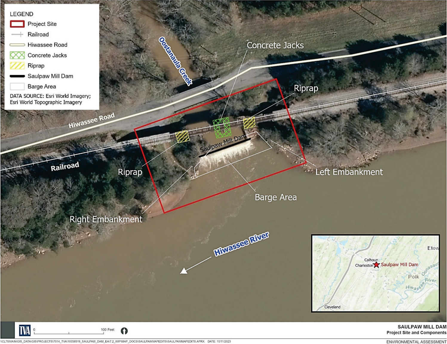
Figure 1.3-2. Saulpaw Mill Dam Project Site and Components
