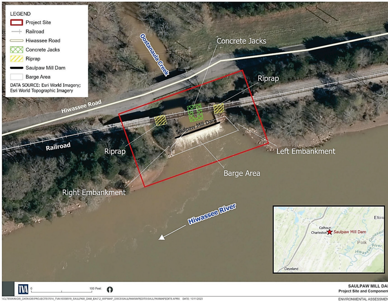
Figure 1-2. Saulpaw Mill Dam Project Site and Components
