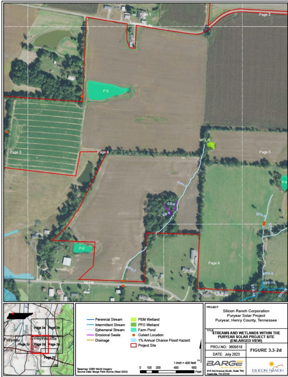
Figure 3.3-2d. Drainages, Streams and Wetlands Within the Puryear Solar Project Site
