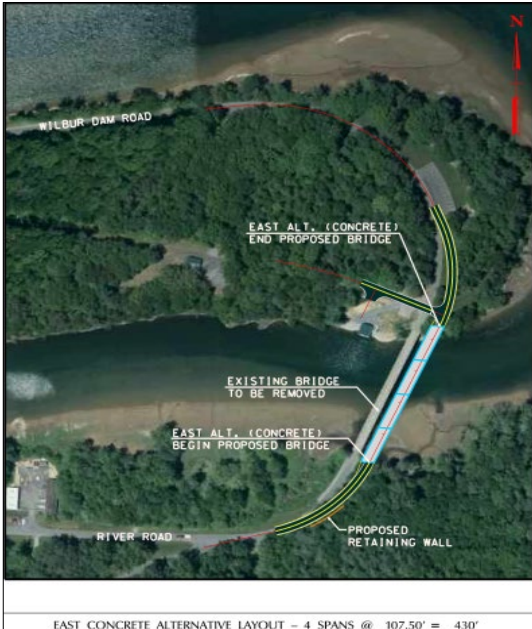
Figure 3. Depiction of a new concrete bridge alternative, aligned on the east side, or just downstream, of the existing Wilbur Reservoir Bridge
