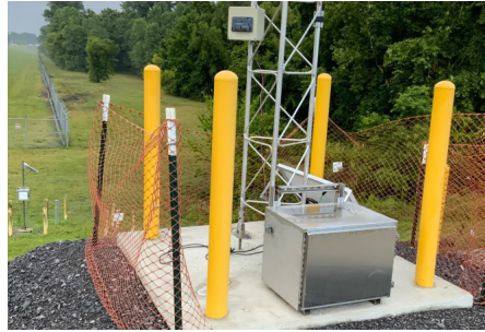
One of 10 air monitoring stations placed around the site that provide continuous readings.
