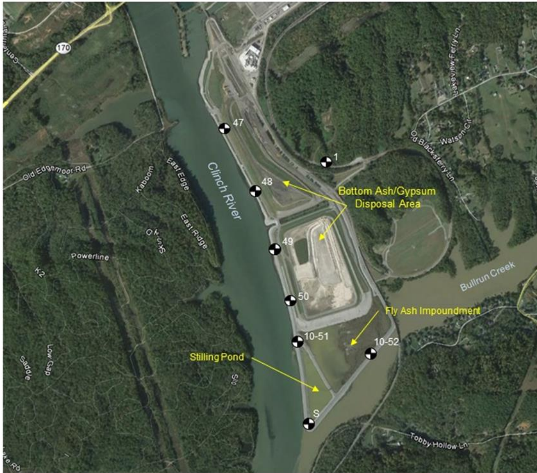
Figure 3-1. Network of Groundwater Monitoring Wells Near Fly Ash Impoundment and Stilling Pond at BRF
