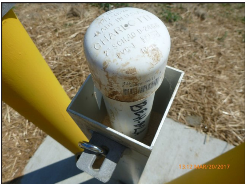
Surface protection for top of well
