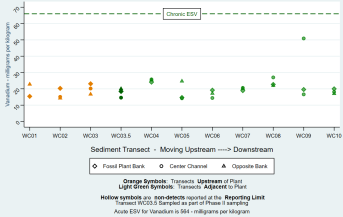
TVA - Cumberland Fossil Plant Vanadium by Transect and Ecological Screening Values (ESVs) for Freshwater Sediment Wells Creek - Sediment
