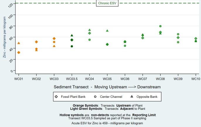
TVA - Cumberland Fossil Plant Zinc by Transect and Ecological Screening Values (ESVs) for Freshwater Sediment Wells Creek - Sediment
