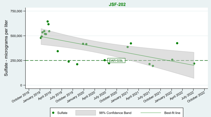
Sulfate - Time Series and Confidence Band John Sevier Fossil Plant - Bottom Ash Pond
