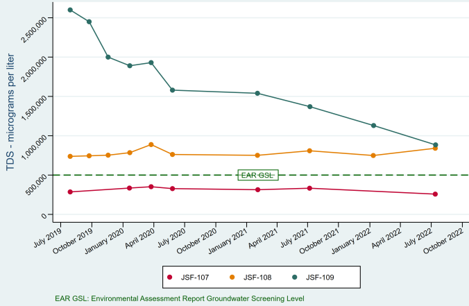
Total Dissolved Solids (TDS) - Time Series John Sevier Fossil Plant - Ash Disposal Area J
