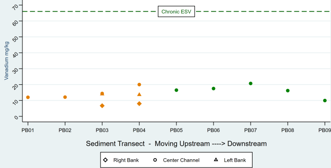
TVA - John Sevier Fossil Plant Vanadium by Transect with Ecological Screening Values (ESVs) for Sediment Polly Branch - Sediment
