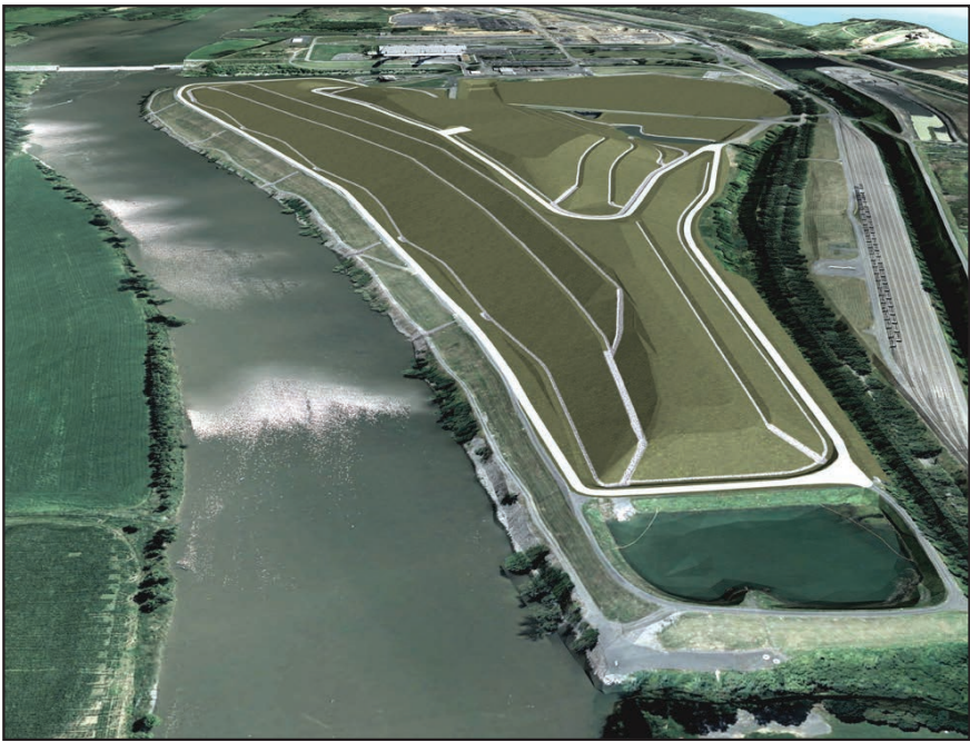
Example of a 3-dimensional model developed and used to calculate volumes
