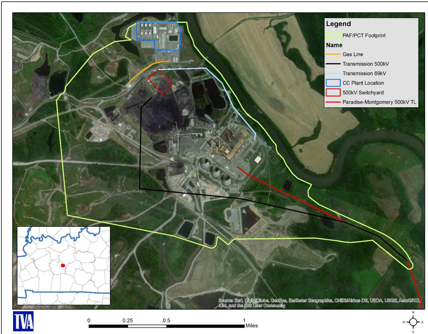
Figure 1. PAF/PCT portion of project footprint. The CC Plant, Paradise-Montgomery 500-kV TL, and 69kV TL are existing. Gas line, 500-kV transmission line, and 500-kV switchyard are proposed.
