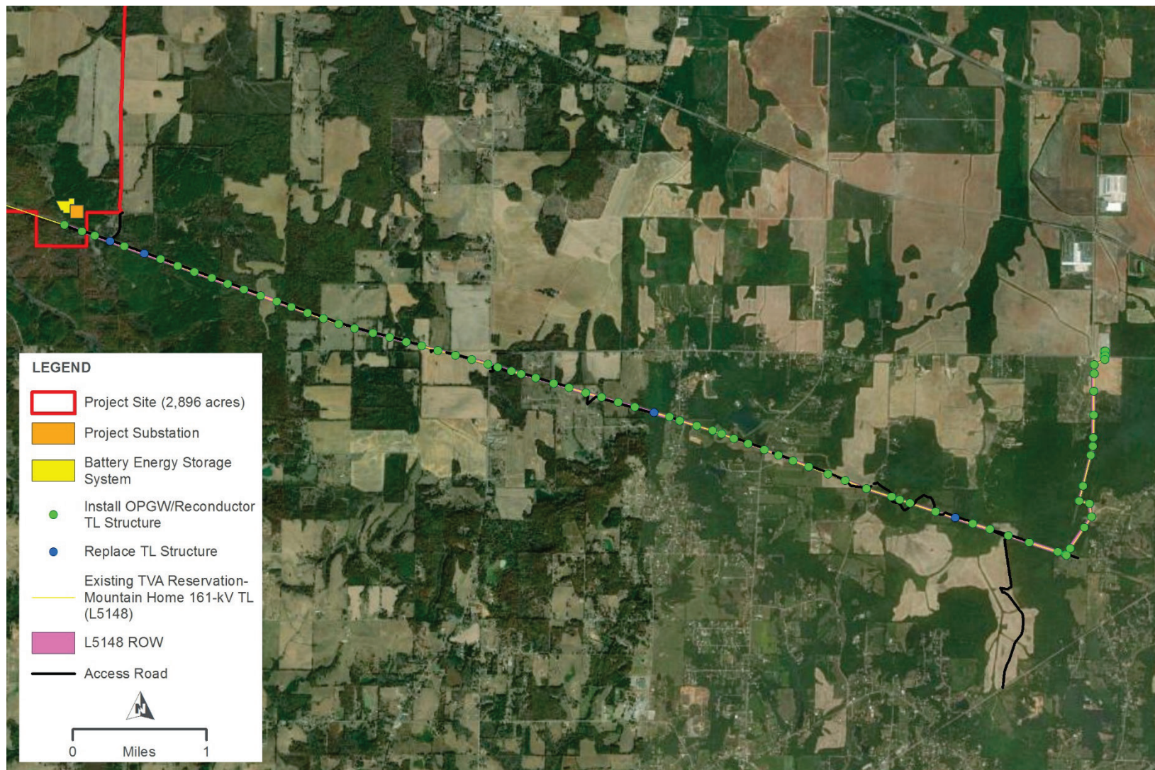
Figure 2-6. The proposed Project substation, battery energy storage system, and work areas along the existing TVA Reservation-Mountain Home 161-kV TL
